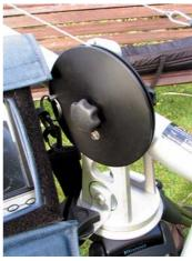
Counter-weights are not supplied so you will need some old gym weights (round centre hole) or similar to counter balance the camera weight. The counterweight bar is not very long so its best to use a selection of weights from 5kg down otherwise you may run out of space on the bar. The crane also has a 'hanging bag' to allow for fine trimming weights to be either hung or placed in the bag. With some trial and error you can work out the counter-weight required for your camera to balance properly.
