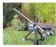
release camera plate to the crane camera plate as I was not happy with the single screw holding my camera to the crane camera plate, plus the obvious advantage of moving the camera between the crane and handheld use.
